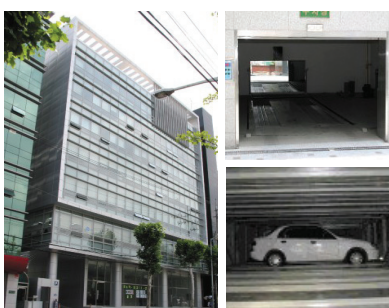
Box parking (Puzzle type with multilevel)
